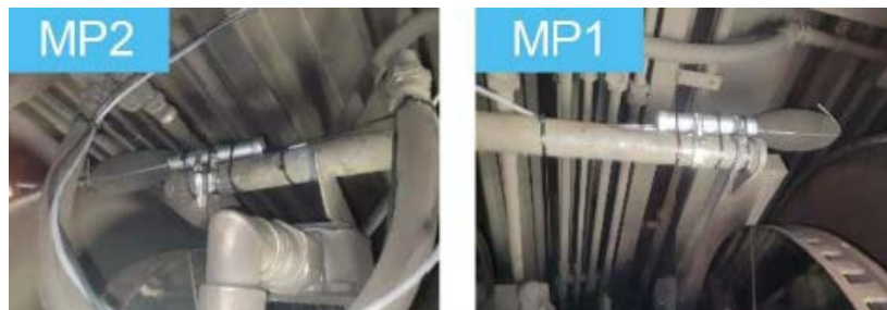
Figure 2-11: On-board microphones for testing acoustic roughness measurements [6]
