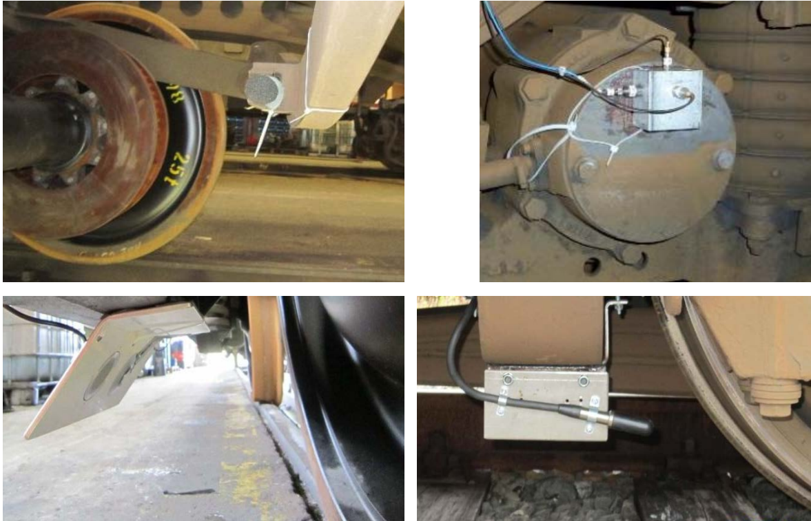
Figure 2-3: SWECO On-board measurement system [6]
