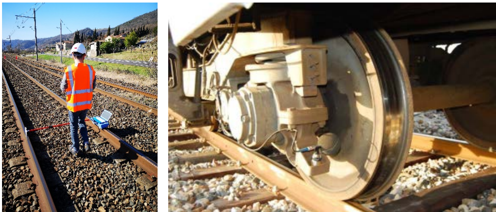
Figure 1-5: Rail roughness measurements - direct (left), indirect (right) [Credit: Vibratec]
