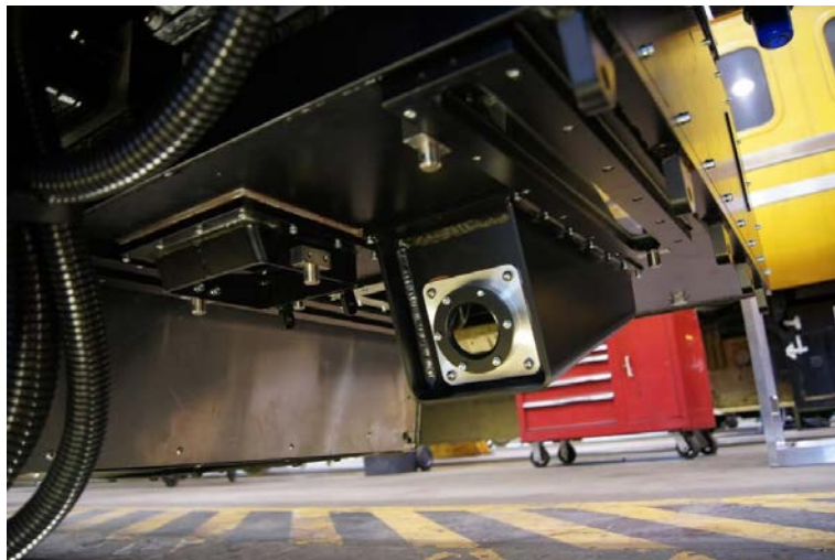
Figure 2-9: NMT sensor setup [Credit: Network Rail]
